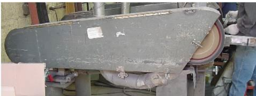
Figure 1 Cover for pinch point hazard
