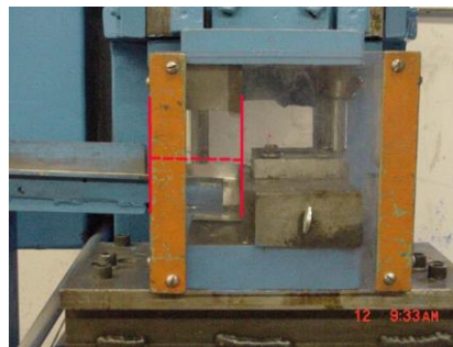
Figure 3 Distance measurement from guard opening to point of operation hazard
